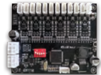
N1042802 12 CH Lock Control Board RS485 Protocol
